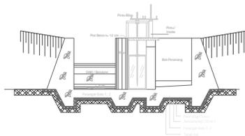
Figure 3 Intake, Settling Basin, Head tank and Spillway.
