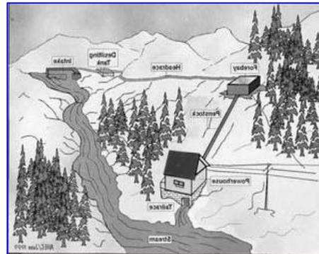
Figure1. Micro hydro Power Plant Components.
